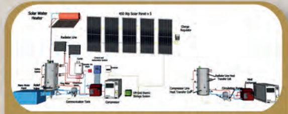
TURKPATENT Application number 2024/000689 "Integrated compressor waste heat recovery system supported by solar generated heat and electricity"
